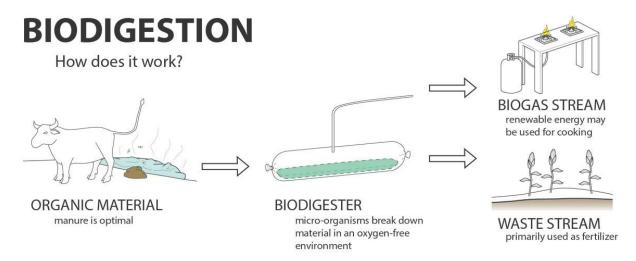
All anaerobic digesters perform the same basic function. They hold manure in the absence of oxygen and maintain the proper conditions for methane forming microorganisms to grow.
