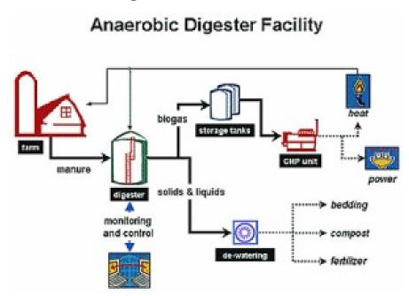
Basically, anaerobic digestion is the process where plant and animal material is converted into useful products by micro-organisms in the absence of air.
