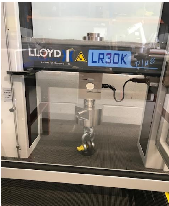
Figure 4: Tensile testing machine
