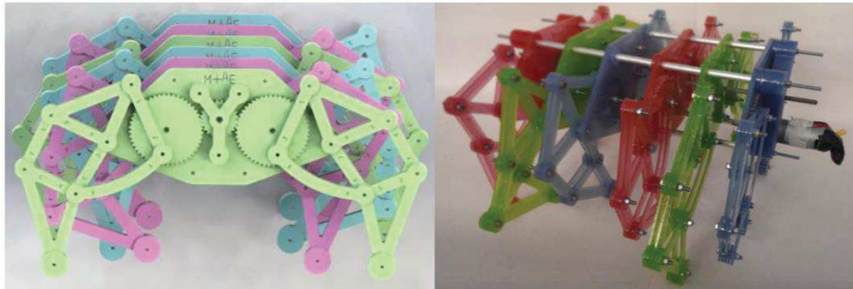
Figure 1: CAD of finalised walking machine design with single motor drive (at rear) showing the redesigned gear train (left) and image of completed walking machine assembly with dual drive capabilities (motors attached at each end).
