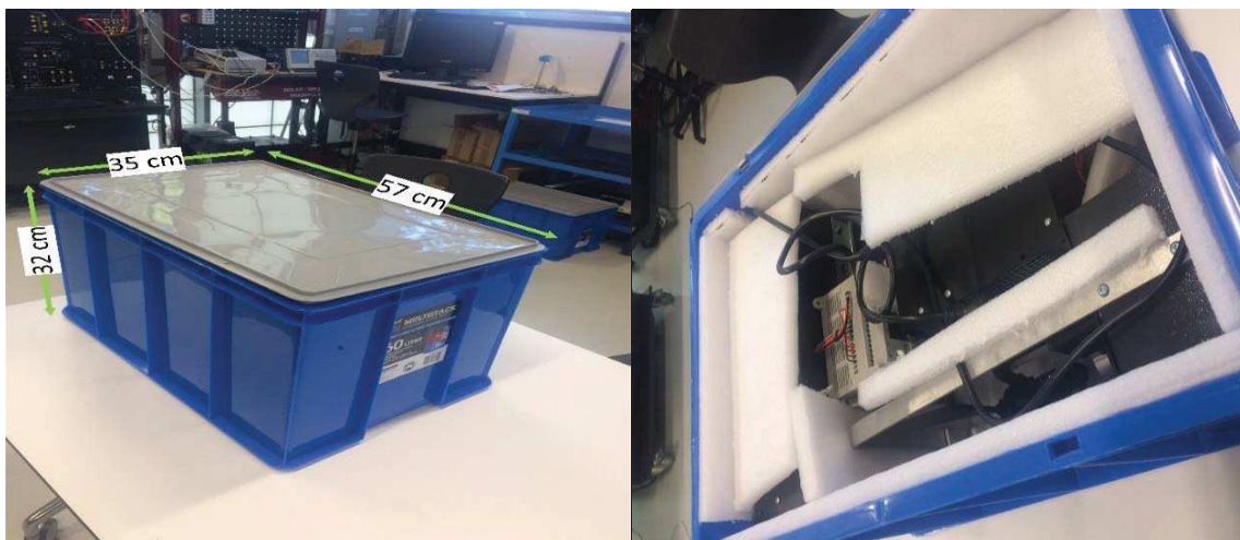
Figure 2: The platform is fit into a portable box (left: the dimension of the box, right: devices arranged in the box).
