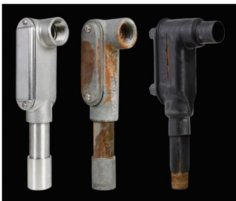
Figure 4: The surface changed due to corrosion
