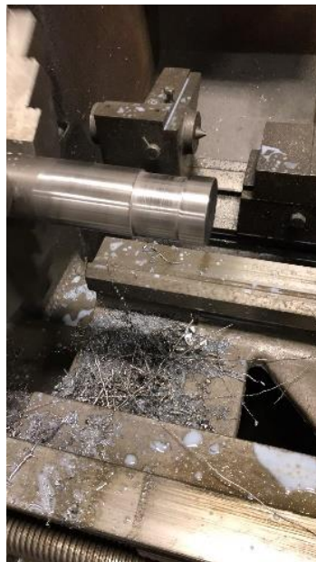
Groove on cylinder being machined. Foster Engineering. being heavy fabrication do not have boring too for small dimension so, Boring process and tapping done at WINTEC.
