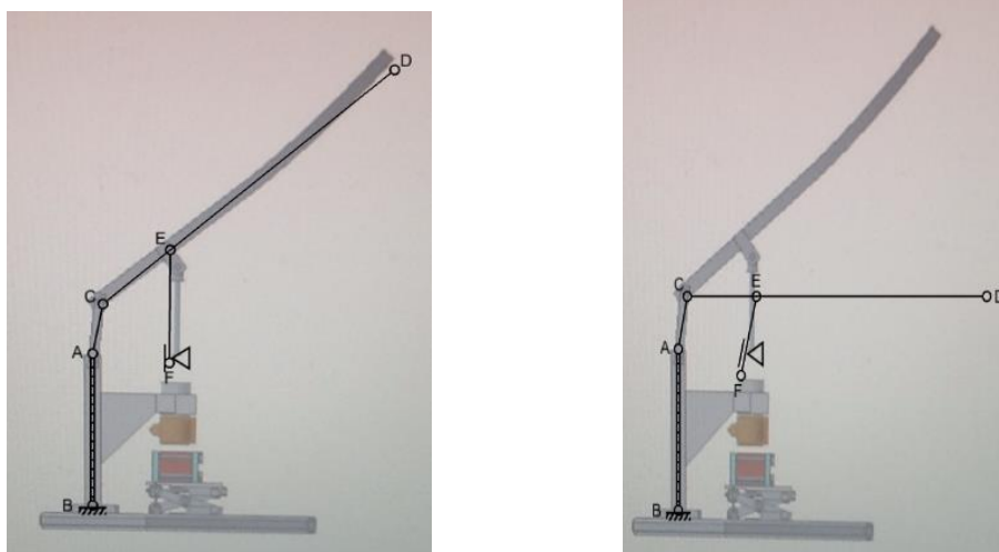
Figure 12. Different length configurations were analysed using Autodesk's ForceEffect Motion. looking into reduce the turning effect in link EF. Angles were
