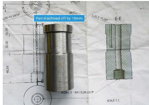
Cylinder compared to 1:1 scale drawing. Part machined is off by 10 mm
