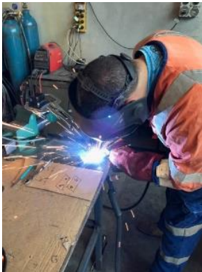
On the left Welding of the clamping clamp. On the centre view of the clamp system. On the right thread tapping of the bracket front plate.
