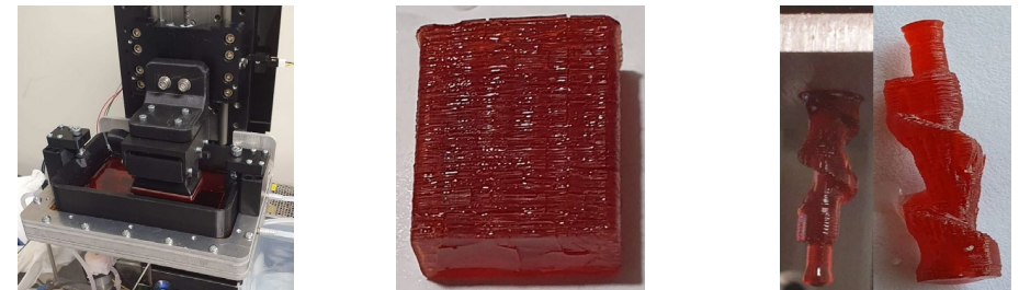
Fig. 1- Interface temperature control 3DP system and printed samples.
