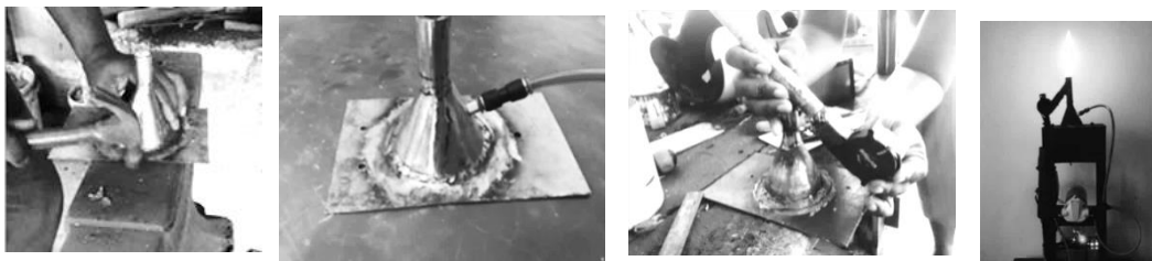
Figure 2: Fabrication of the funnel, Nozzle connection, Blower Connection, Complete assembly of standalone gassified liquid burner in operation.
