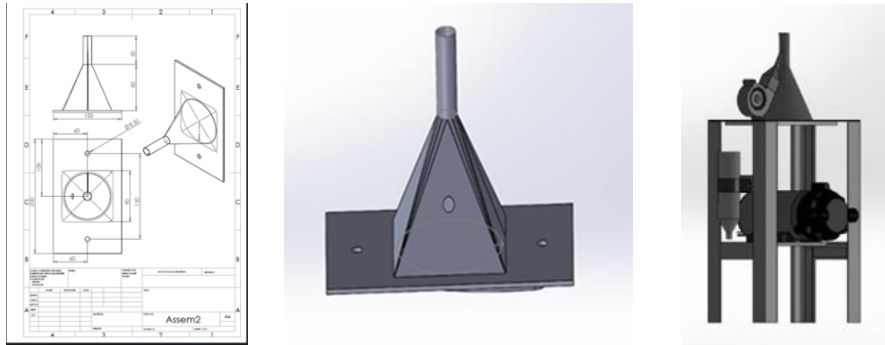
Figure 1: Drawing of the funnel and the sub system assembly and structure
