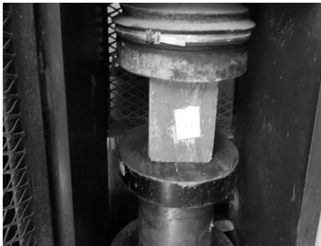
Figure 1: Compressive Strength Testing for Cube
