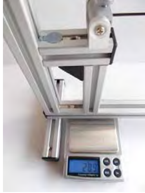
Figure 6: LHS reaction measurement
