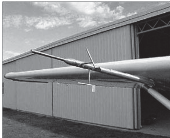
Figure 2: The air-data boom mounted on the starboard wing.
