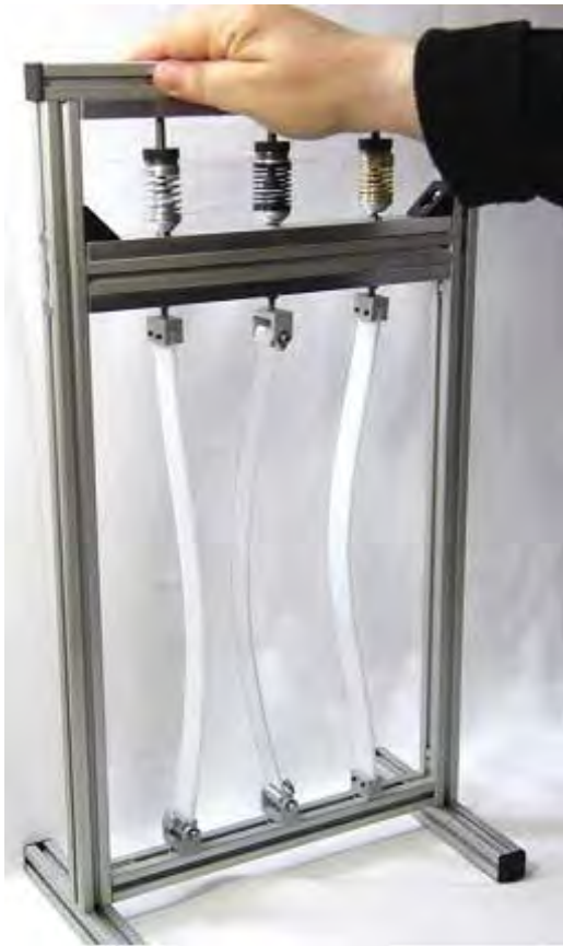
Figure 14: Column Buckling: Fixed-Pinned; Figure 15: Column Buckling: Fixed-Fixed Roller; Pinned-Pinned; Fixed-Fixed Fixed-Pinned Roller (Sway cases)
