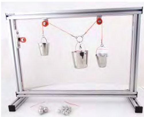
Figure 13: Equilibrium of co-planar forces (300, 500, 400 g case and all 300g, respectively)
