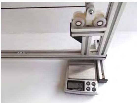
Figure 8: Tare function “zeros-out” to the ‘no load’ reading for RHS reaction absolute
