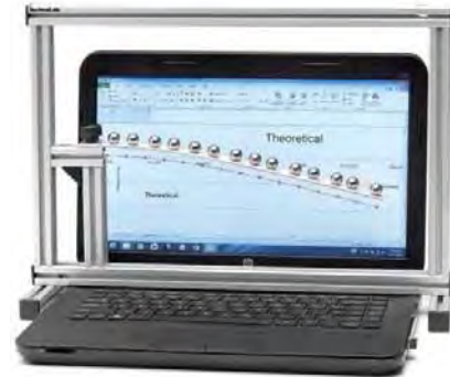
Figure 2: Pixi Frame with Notebook Prediction Cantilever Expt.
