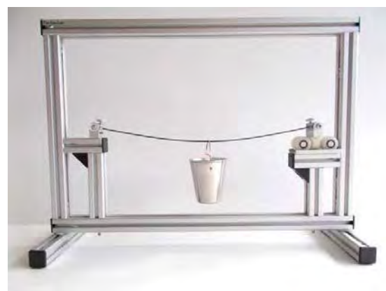
Figure 4: Simply supported CF beam central point load
