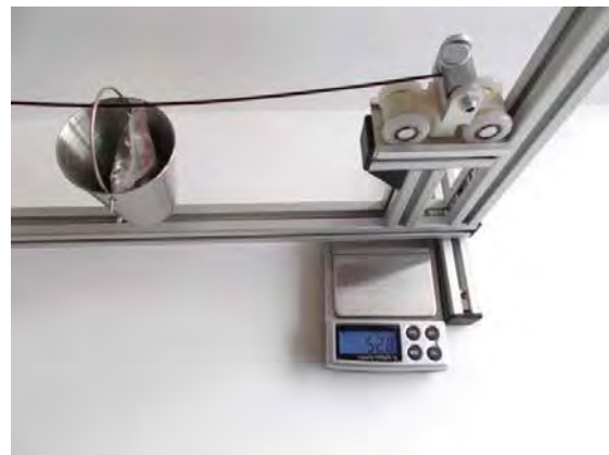
Figure 9: RHS reaction measurement applied load is now
