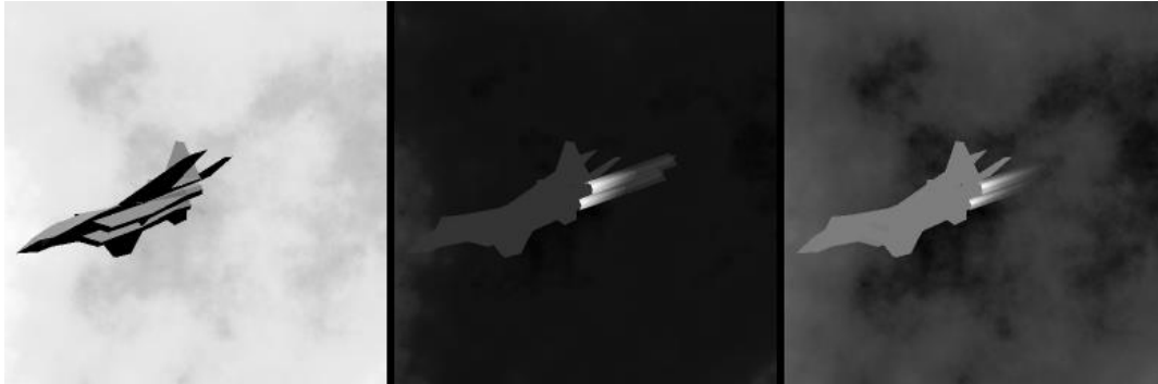
Figure 6: Calculated signature images in the near infrared, the 3-5 \mu\text{m} and the 8-12 \mu\text{m} spectral bands.
