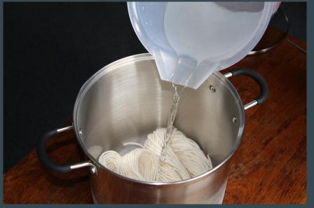
Energy use is tracked per dye bath, this enables comparisons to be made. 100% New Zealand wool year is weighed out, covered with water and left to soak overnight. By soaking the yarn before dyeing it the yarn is able to uptake the dye easier, eliminating the need for Lyogen (a chemical used to help yarn absorb dye).
