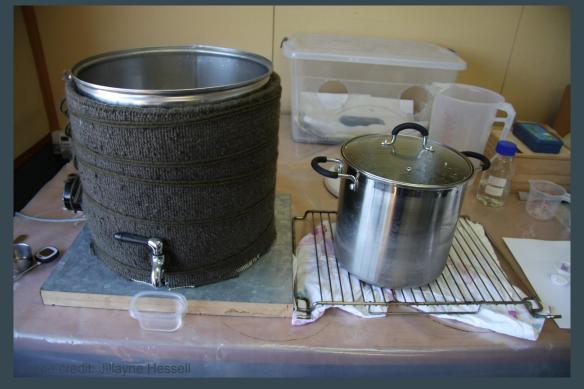
Equipment for the dyeing process is set out as above. A bain-marie type system is used to heat and control the temperature of the dye bath.
