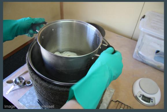
To avoid unnecessary energy loss the outside of the bain-marie is wrapped in a wool rug. New research suggests colouration factories continue looking at ways to insulate and contain heat already produced.
