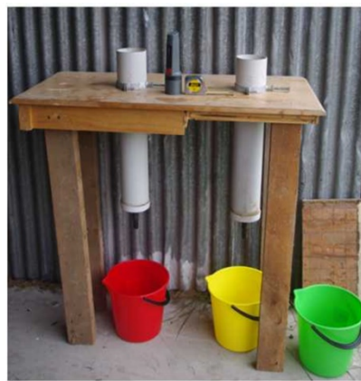
Figure 1. 'Bucket science' measurement of saturated hydraulic conductivity by falling head permeameter.
