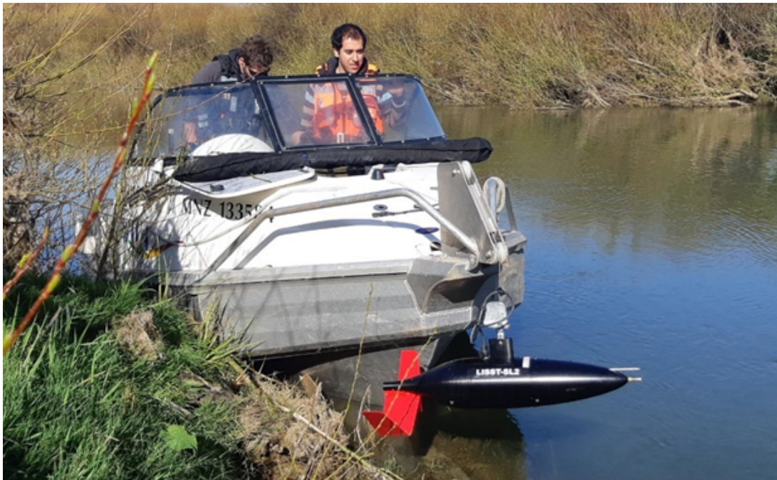
Figure 1: LISST-SL2 deployed from a jetboat on the Oreti River at 29 m 3 /s.
