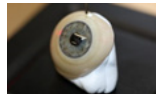
Measuring the surface hydrophilicity of a prosthetic eye
