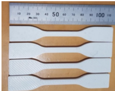
Figure 1. ASTM type IV printed ABS tensile samples, printed at different layer heights ranging between (top) 0.2mm – (bottom) 0.8mm.
