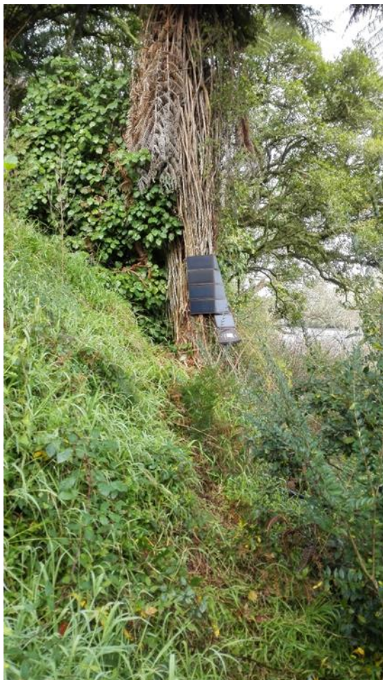
Figure 2: This shows the physical location of the Cacophony Bird Monitor that was used to capture the recordings for this work. The Bird Monitor is inside a waterproof box behind the solar panel that can be seen attached to a fern tree.
